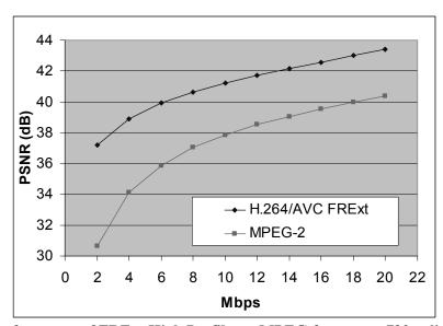
Fig. 9: Objective Performance of FRExt High Profile vs. MPEG-2 on a test 720p clip "BigShips". (These objective results are consistent with the subjective results in Fig. 8, i.e, 8 Mb/s of FRExt outperforms 20 Mb/s of MPEG-2.)
