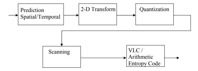
Fig. 2: Higher-level encoder block diagram
