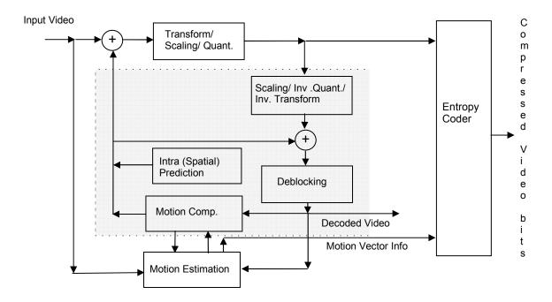
Fig. 1: High-level encoder architecture
