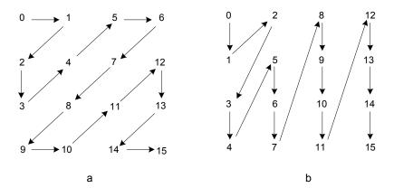
Fig. 4: Coefficient scanning order in (a) Frame and (b) Field modes
